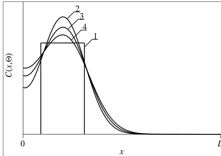
**Fig 3b:** Spatial distributions of dopant in heterostructure after ion implantation. Curve 1 is idealized distribution of dopant. Curves 2-4 are real distributions of dopant for different values of annealing time. Increasing of number of curve corresponds to increasing of annealing time
