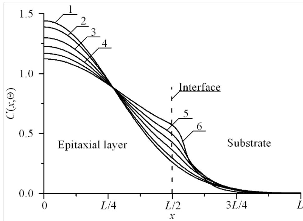
**Fig 2a:** Distributions of concentration of infused dopant in heterostructure from Figs. 1 and 2 in direction, which is perpendicular to interface between epitaxial layer substrate. Increasing of number of curve corresponds to increasing of difference between values of dopant diffusion coefficient in layers of heterostructure under condition, when value of dopant diffusion coefficient in epitaxial layer is larger, than value of dopant diffusion coefficient in substrate
