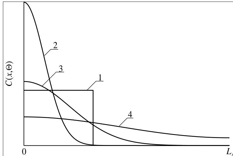
**Fig 3a:** Spatial distributions of dopant in heterostructure after dopant infusion. Curve 1 is idealized distribution of dopant. Curves 2-4 are real distributions of dopant for different values of annealing time. Increasing of number of curve corresponds to increasing of annealing time
